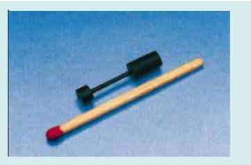
Figure 58 A Ceramer cylinder machined on a lathe.
